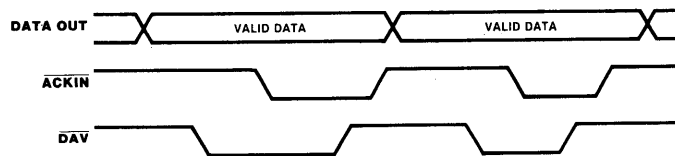
Figure 5. Two-Wire Interlocked Handshake Timing (output)
